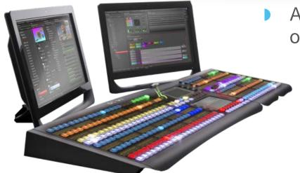
All functions can be controlled by one or multiple GUI's, or via built in touch screens
