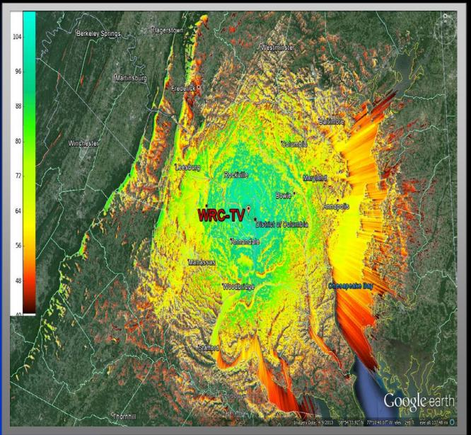
DC – WRC-DT (ATSC 3.0 1 MW ERP on Ch. 36)
