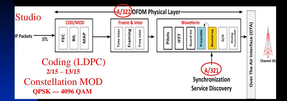
Time /Frequency Interleaving Cell Multiplexing
