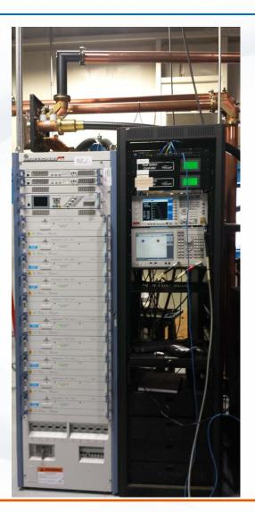
At Dielectric Factory at 9kW ATSC and 9kW DVB-T (6 MHz)
