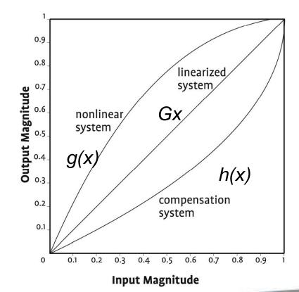
An amplifier characteristic g(x)may be corrected for with a complementary characteristic h(x)such that g(h(x)) = Gx
