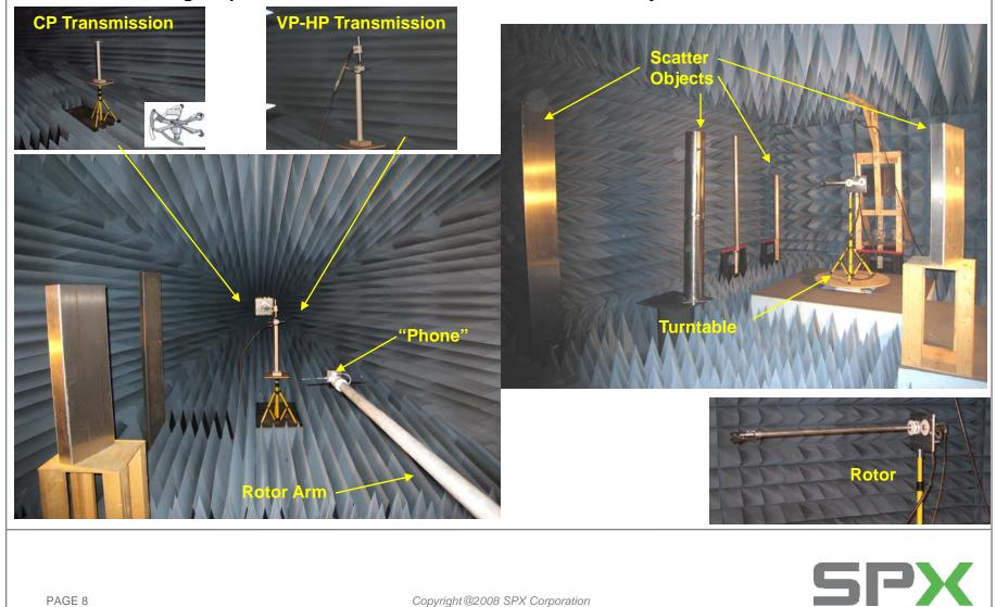
Both polarization mismatch and small scale fading produce variability in the signal as the receiver changes orientation and location
