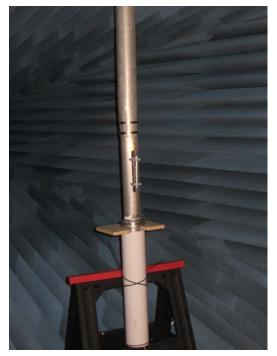
Elliptically polarized transmit antenna
